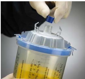
After shaking, check lid and tighten if needed. Allow paint to settle and slowly remove plug to release any air.
