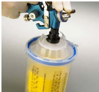
Mount the adapter flush to the lid tower base by pressing down firmly on the spray gun.
